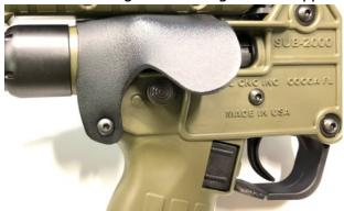
Step 3: Work quickly to shape Kydex to desired position. You can re-heat as needed to continue shaping the Kydex Shell Deflector.
