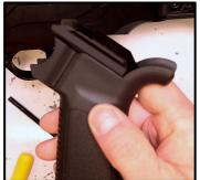
Step 7: Tap the Trigger Guard with your Palm a few times to Remove it from the Chassis.
