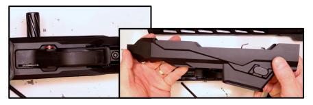
Step 8: Make sure your Bolt is Forward, Then use your 1/8" Punch to Push Out the Two Takedown Pins Near the Trigger Group.
