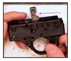
Step 11: Insert the First Small Pin in the Hole near the Bolt Stop. Make sure it is even with the Raised Portion of the Trigger Group.
