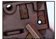
Step 12: Use your Stainless Steel Pin to Push Out the Factory Hammer Hinge Pin.
