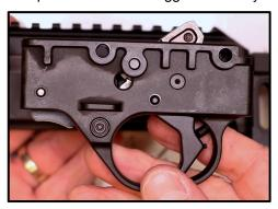
Step 10: Place the Assembly on Fire and Let your Hammer Forward.
