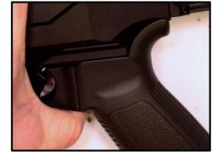
Step 20: Keeping the Grip in Place, Drop in the Long Rear Takedown Pin through the Top and Tighten it with your 5/32" Allen Key.
