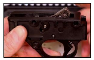
Step 15: Turn the Receiver Upright. Make sure the Bolt is Forward and Drop in the Trigger Group.
