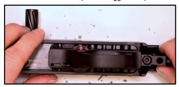
Step 16: Line up the Trigger Group with the Holes on the Receiver.
