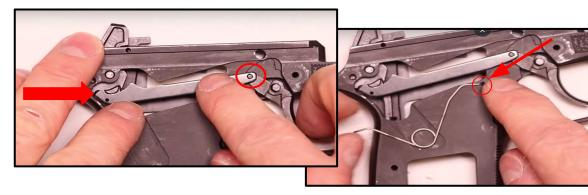
Step 26: Now take your index finger and hold down the coiled part while pushing up on the short leg until you can hook it into that hole. The tension will hold everything in place.
