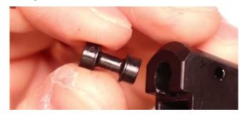
Step 24: Using your hammer, lightly tap the pin into place.
