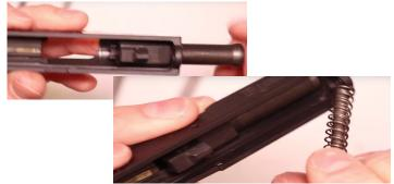
Step 19: You will need to remove the torx screws and panels from each side. Then begin to remove the factory trigger return spring and trigger bar.
