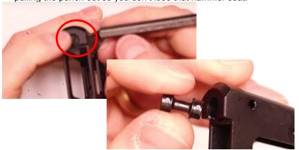
Step 22: Now let your hammer spring slide out and replace it with your new M\*CARBO hammer spring, swapping the hammer spring **guide** into the new spring as well.
