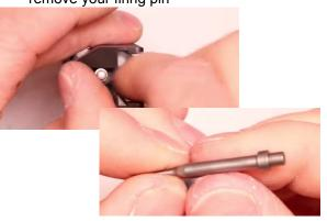
Step 12: Set your firing in to the side and slide out your firing pin spring.
