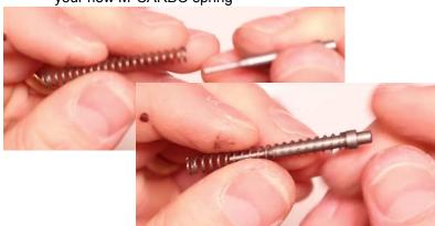
Step 14: Slide your firing pin and firing pin spring back in. You will need to compress it with your ½ punch while sliding the plate back into place.
