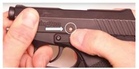
Step 4: Turn the gun on the other side and with your 1/16 inch punch and push the pin out.
