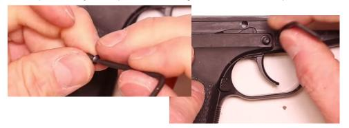
Step 29: Flip your firearm to the other side, make sure the slide stop spring is in place and that the spring locates in the small hole on the slide stop.
