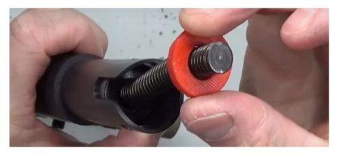
**Step 6**: Put the buttstock back on, Place the hard plastic buffer at the end. Line up the holes to put the buttstock pin back in place.
