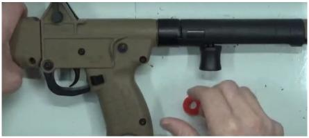
**Step 2**: Fold your Sub 2000 in half. Press down on the hard plastic recoil buffer. Then pull out that buttstock pin.
