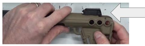
**Step 5**: Slide the Recoil Buffer over top of the recoil spring inside of the receiver tube. Pull the charging handle to bring it down.
