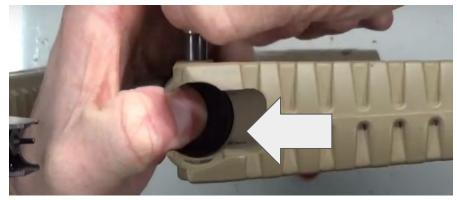
Step 3: Remove the hard plastic buffer and the buttstock
