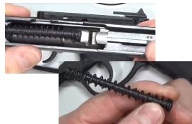
Step 6: Remove the factory guide rod from the springs, making sure the smaller one stays in the middle. Then replace that rod with your new M\*CARBO Guide Rod.
