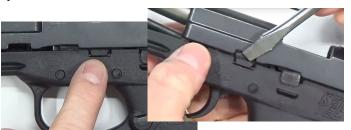
Step 4: Lock the slide back, and remove the take down pin.
