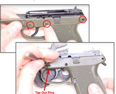
Step 23: After you've removed those frame pins, set them to the side. Now pull back on the trigger just a hair while pulling up on the aluminum frame. Pinch the front portion of the frame while you are pulling it out to keep all that linkage together.
