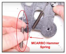
Step 37: Take your 3/32 Punch to press down and then use your Hammer to tap out the Hammer Spring.
