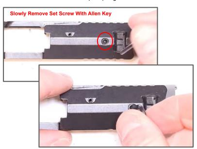
Step 10: Do not fully unscrew the set screw. Take your ½ inch punch and set it in front of that firing pin, this way you won't lose any components. You should have to back out a couple threads to get the firing pin out.
