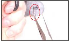
Step 33: Once the Pin is removed, you should be able to pull the Trigger Return Spring right out.
