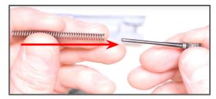
Step 12: Now you will put your firing pin and firing pin spring back into place. Make sure that set screw is lined up with that notch and the smooth side is facing you.
