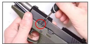
Step 4: Set the assembly pin off to the side and remove your slide from the frame.
