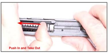
Step 7: Remove the barrel.
