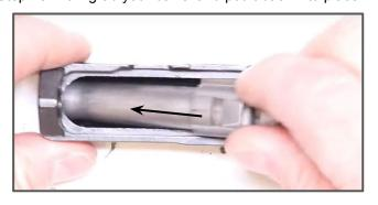
Step 19: Then you can take your recoil spring and guide rod, push them forward making sure it locates on both the nose of the slide and on the lug.
