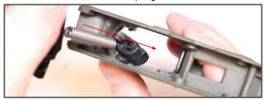
Step 59: Now rotate the Aluminum Frame and compress it onto the Pistol Grip Frame.
