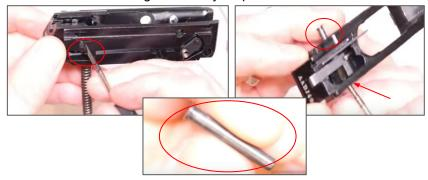
Step 29: Then you're going to push out the Hammer Spring.
