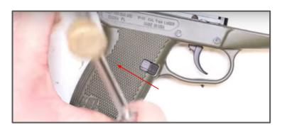
Step 62: Once you got the Pins in the Frame, you're going to set the Spring Tension on the Hammer. Pull up on the Hammer Spring Catch all the way and you want to clear the two little tabs.
