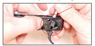
Step 46: Next you're going to insert your Trigger Pin into the Trigger and press it in as much as you can and then use your Hammer to push it all the way in. Use your Bench Block for leverage.
