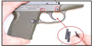
Step 61: Use your Hammer to push the Pins all the way into the Frame.
