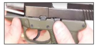
Step 65: Pull back on the Slide Lock and then insert the Assembly Pin.
