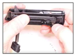
Step 24: Now you will need to exchange your hammer spring out. Make note of the orientation of the spring, both loops are facing the rear of the aluminum frame. The shorter leg goes toward the hammer spring catch & the longer leg goes up on the hammer.
