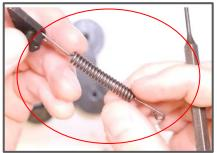
Step 38: Once you remove the Factory Hammer Spring, Grab your New MCARBO Hammer Spring for the install.
