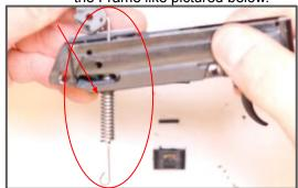
Step 49: Next, line up the Hammer Hinge Pin with the holes and drop it in the Frame.
