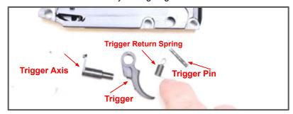
Step 43: Insert your Trigger into the Frame and then drop the Trigger Axis in as well, it should pop right in. Make sure that the holes line up.
