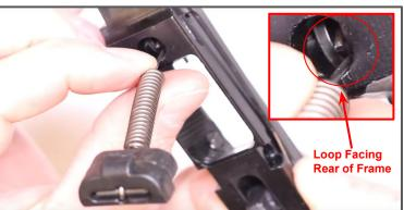
Step 25: Now push down on that hammer spring and remove that hammer spring pin and catch as so:
