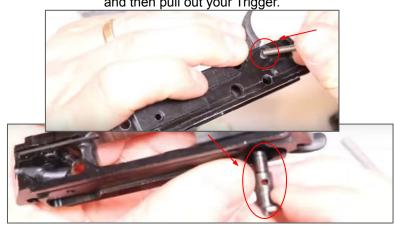
Step 35. Now you should have all of your components removed from the pistol grip frame and it's time to replace the springs and put it all back together.
