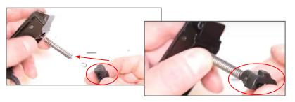
Step 51: Next, you're going to insert your Hammer Spring Pin right through the loop on the Hammer Spring.
