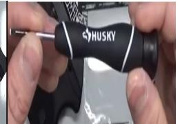
Step 4: Remove factory guide rod from recoil spring
