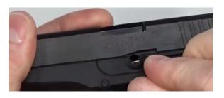
Step 6: Put the slide the back and push back about an eighth of an inch so you can get the takedown pin lined up. Make sure the lugs aren't sticking out and the hole is completely clear
