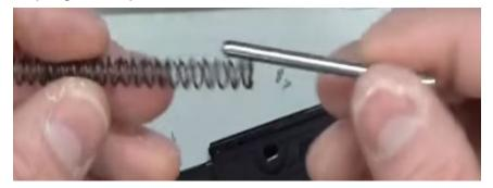
Step 7: Make sure hole is completely clear and go in a 45 degree angle. Hit the spring that is there and push it and it drops right in and lock it back
