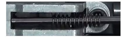
Use the larger Allen Key and slide spring into the hole.
