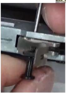
Step 7: Use the 3/32" Punch, press through the hole to remove the Trigger Hinge Pin. Set Hinge Pin Aside.
