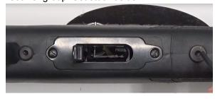
Step 5: Remove the Tape Down Screw Stud. Set aside.
