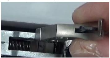
Step 10: Insert M\*CARBO Trigger Return Spring into place. Use the 3/32" Allen Key and place the spring onto it. Insert the end of the Allen key into the hole.
