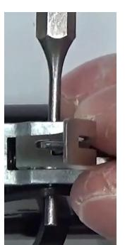
Step 12: Take hinge pin and push onto the punch, and slide Hinge Pin into hole.
