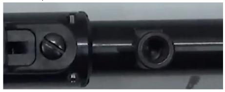
Step 16: Place stock over the receiver barrel.
