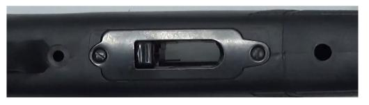
Step 17: Insert screws. Place shortest screw in front and longest screw in rear.
