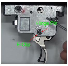
Step 6: Focus on the trigger assembly. Remove E-clip using the Flat-Head Screwdriver.
