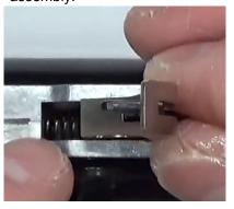
Step 12: Insert the 3/32" punch into the Hinge pin hole.
