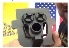
Step 4: Finally make sure the Vise Block is compressed on the Muzzle Plate creating a nice solid steel on steel lock.
