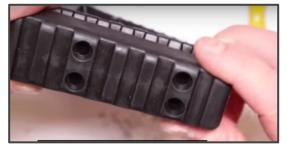
Step 10: Continue drilling until holes are matched up and cleaned out.
