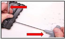
Step 17: Take one of your Countersunk Screws and start hand screwing it to get it started along with the 3/32 Allen Key on the other side.
