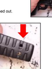
Step 11: After you're finished with the holes, it should snap on nice and solid. It is adjustable, so if you experience some resistants, you can use your drill and clean up the hole.
