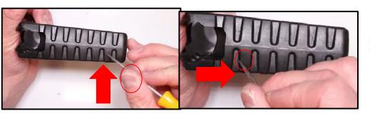
Step 7: Hold the Buttstock at an angle and then take your ½ inch drill bit and hold that at an angle as well and drill where you made the little dots.
