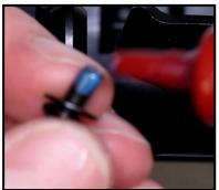
Step 11: Use your 3/32" Allen Key to Tighten the Screw back onto the Sling Mount.
