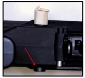
Step 10: Grab the Sling Mount Screws and put some Blue Loctite on the Threads.
