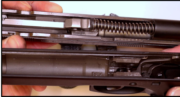
Step 6: Compress and Pull Out the Guide Rod and Recoil Spring.
