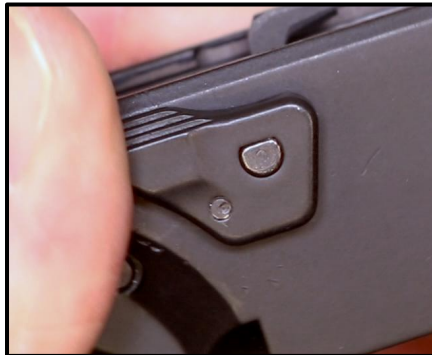
Step 66: Attach the Other Side of the Decocking Lever. Hold it down and Use your Micro-Tip to Pull down the Inner Pin.
