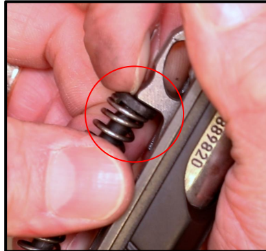
Step 6: Compress and Pull Out the Guide Rod and Recoil Spring.
