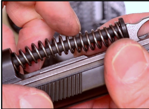
Step 6: Compress and Pull Out the Guide Rod and Recoil Spring.
