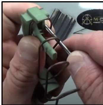
Step 6: Use your Punch to help Remove the Factory Spring from the Follower.
