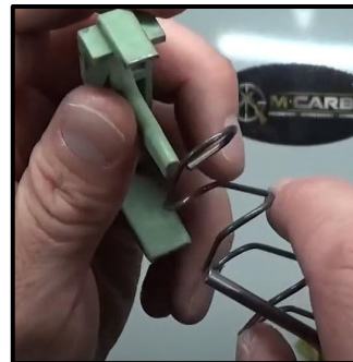
Step 8: Reinsert the Follower and Mag Spring into the Magazine from the Bottom
