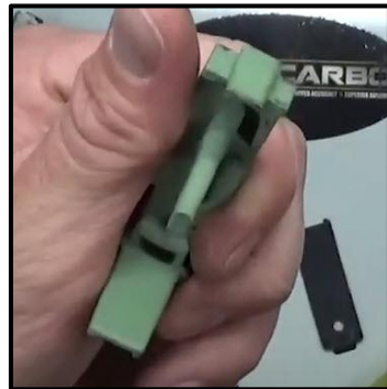
Step 6: Use your Punch to help Remove the Factory Spring from the Follower.
