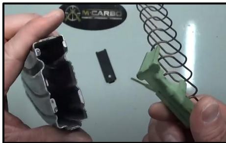
Step 6: Use your Punch to help Remove the Factory Spring from the Follower.
