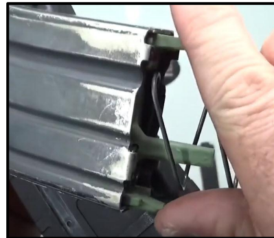
Step 8: Reinsert the Follower and Mag Spring into the Magazine from the Bottom
