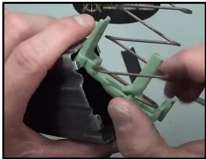
Step 6: Use your Punch to help Remove the Factory Spring from the Follower.
