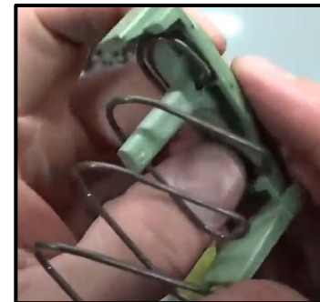
Step 8: Reinsert the Follower and Mag Spring into the Magazine from the Bottom
