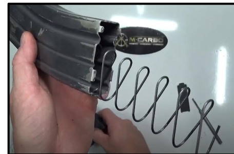
Step 8: Reinsert the Follower and Mag Spring into the Magazine from the Bottom
