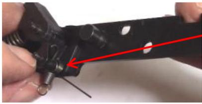
Step 12: Place the sear, sear spring and the coil spring on the post beneath the hammer.
