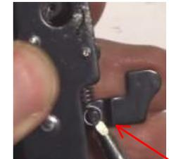
Step 20: Place extension spring on post of bolt release lever.
