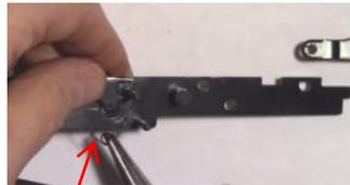
Step 6: Remove the stock disconnecter spring
