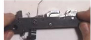
Step 17: Put top plate back on and reinstall the 3 e-clips to hold it in place.
