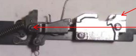
Step 15: Place feed ramp & linkage back in position.
