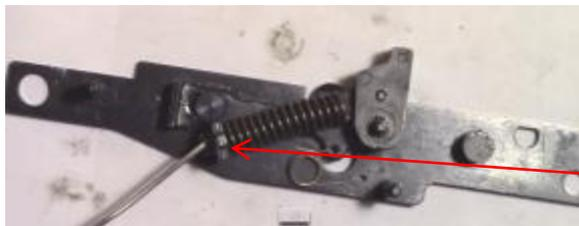
Step 11: Drop hammer back onto post on the plate. Make sure the notch drops into the hole on plate.
