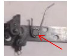
Step 14: Put the extractor spring on the large post.
