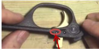
Step 1: Press out the forward pin on the trigger guard; from right to left or towards the red on the safety button
