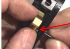
Step 2: Insert the M-CARBO trigger return spring and re-insert the pin.
