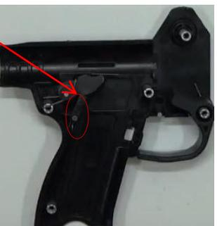
Step 18: Place MCARBO Sear Spring onto sear. Short leg on top of sear and long leg behind stud.
