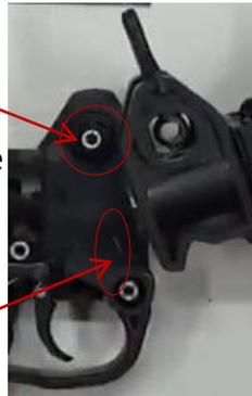
Make sure tab on sear sticks through this cut-out on trigger bar.
