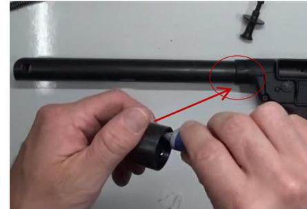
Step 36: Insert charging handle into hole in bolt. Then insert recoil spring all the way into receiver.
