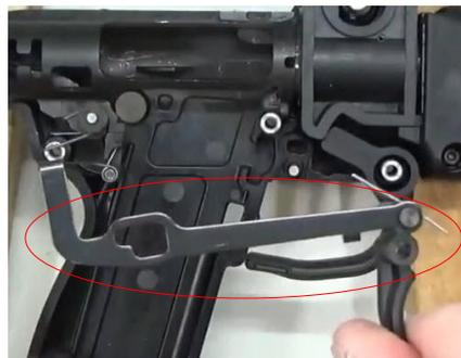
**Step 9:** Remove Trigger, Trigger Return Spring and Trigger bar by pulling up carefully on the trigger.
