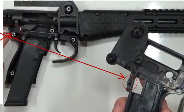
Step 25: Insert Magazine release into this hole.
