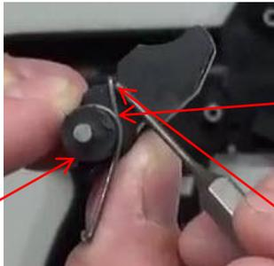
Make sure this straight leg is above the hinge pin and the loop of the hammer spring is behind the strike face.
