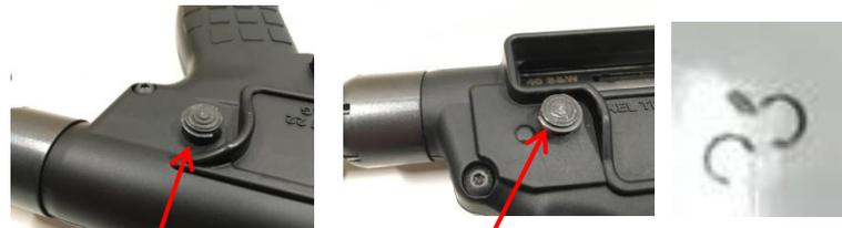
**Step 3:** Remove the 2 c-clips from both sides of the cross bolt safety. The detent will also fall out once clips are removed.
