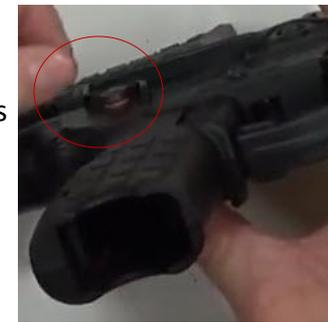
Step 34: Re-insert Bolt. Keep hole on bolt lined up with track on receiver.
