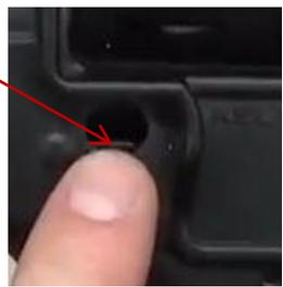
Step 31: Insert punch from left side and insert safety from right side. Make sure "Fire" side of safety is on the right side. Use punch to push down on trigger bar.
