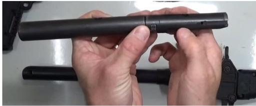
Step 35: Install Castle Nut (collar). Apply Loctite to inside of Castle Nut (collar) and twist onto trigger housing.
