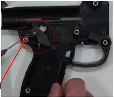
Step 17: Insert Sear and stage hammer in this position on top of sear. Leave hammer in this position for remainder of install.
