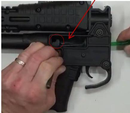
Step 28: Re-insert all 10 screws into trigger housing. There are 5 on each side. Don't over tighten.
