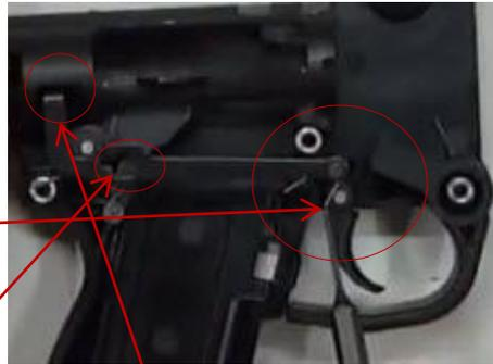
Step 23: Test to make sure trigger bar moves up and down.
