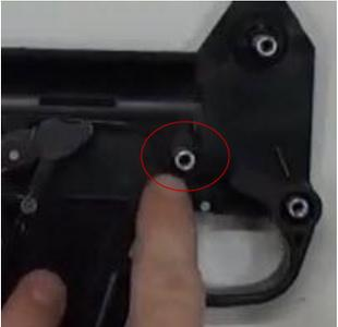
Step 20: Insert Receiver into trigger housing. Line up tabs on receiver with cut outs on trigger housing. Re-install stud you removed from step 19.
