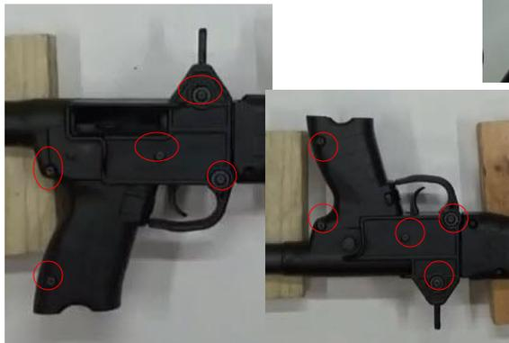
**Step 4:** Remove all 10 screws from trigger assembly. 5 screws on each side.
