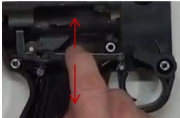
Step 24: Re-Install barrel by inserting barrel over stud and lining it up with hole in the sight. Also make sure barrel stays in front of this spring as it should provide tension.
