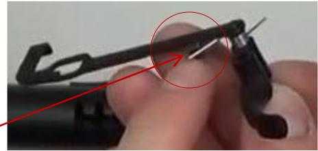
Step 22: Re-Insert Trigger into trigger housing. Then move short leg of trigger return spring clockwise around and over the trigger hinge pin on the trigger housing to provide necessary tension.
