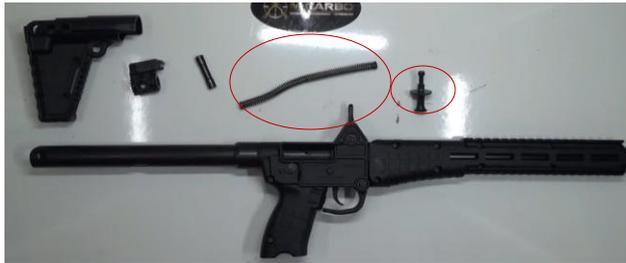
Step 37: Lastly, Insert buttstock, buffer and pin in that order. Then perform a function check.
