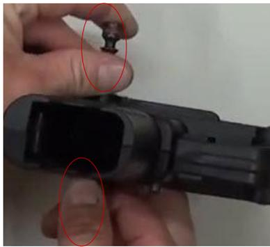
Step 32: Insert detent into small hole on safety. Use razor blade to compress detent and insert the safety back into the trigger housing. Don't push it too far back inside.
