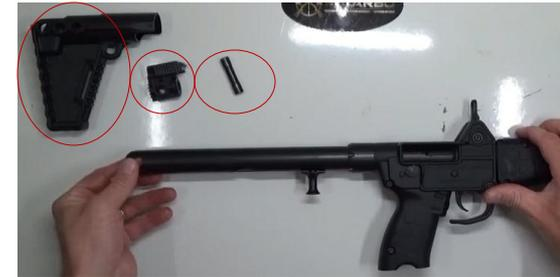
**After you have reassembled your KEL TEC SUB-2000 make sure you do a function check.** Cycle the action and load a snap cap or spent shell casing into the chamber. With the rifle safety on "safe" and the barrel pointed in a safe direction, verify that the rifle will not fire when you attempt to pull the trigger. Place the safety now on "fire" and now verify the hammer falls.
