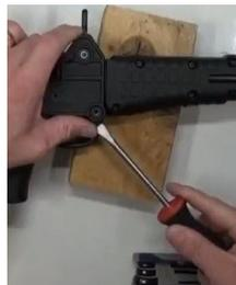
**Step 5:** Carefully pry apart polymer plastic trigger assembly.
