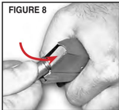
• Inspect your pistol as previously described in the “Inspecting Your Pistol” section. Hold the pistol in one hand with the muzzle pointing in a safe direction and with your finger off the trigger and outside the trigger guard. Insert the loaded magazine into the magazine well (opening) of the pistol until it is locked in place.
